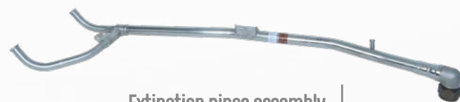
Extinguishment pipes assembly A320 – AIRBUS ATLANTIC
