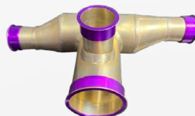
Assy tube welding fuel system CHALLENGER 300 – BOMBARDIER
